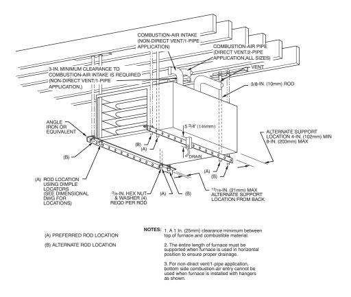
Fig. 22—Crawlspace Horizontal Application
